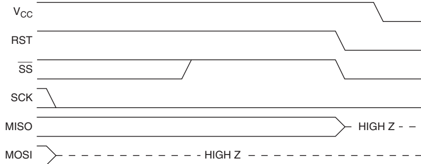
Figure 22-23. Serial Programming Power-down Sequence
